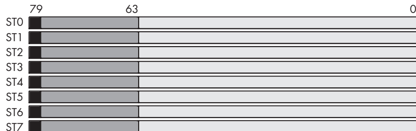
Figure 6-1: FPU floating-point register stack
